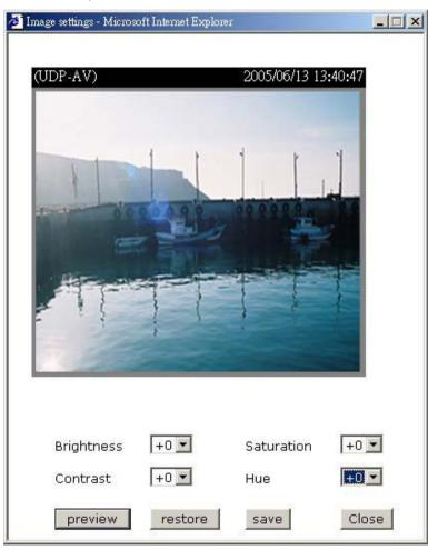
levels ranged from -5 to +5. In "Brightness" and "Contrast" fields the value 0 indicates auto tuning. The user may press Preview to fine-tune the image. When the image is O.K., press Save to set the image settings.
